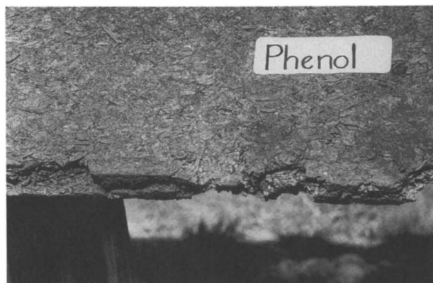
Figure 4. Photographic comparison of 12 mm thick exterior grade commercial particleboards manufactured in the same industrial plant and bonded with MUF, wattle tannin-formaldehyde, and PF resins. The panels were exposed at the CSIR testing site (4,500 feet above sea level) at Pretoria, South Africa for 15 years. Note the extensive degeneration of MUF board (commercially imported MUF resins from West Germany). Also note the more marked edge and surface degeneration of the PF in comparison to the TF-bonded boards.
